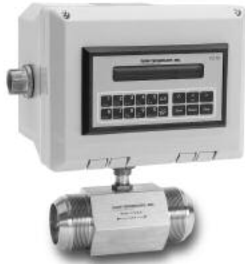
The FC70A-B1-A6 is shown mounted directly on a Flow Technology 2-inch turbine flowmeter. The FC70A is housed in a NEMA 4X/IP65/Exn enclosure with two conduit hubs. The enclosure is also available with MS connectors for cable connections. The FC70A panel mount configuration has a watertight seal which meets NEMA 4X/IP65 standards.
